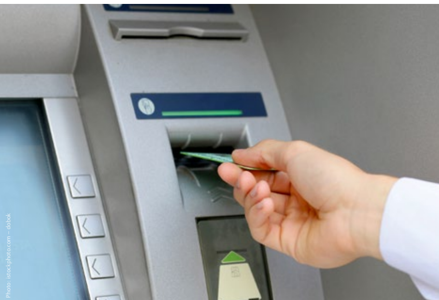
Cashpoints are programmed so that the money can only be drawn once the card has been taken.
