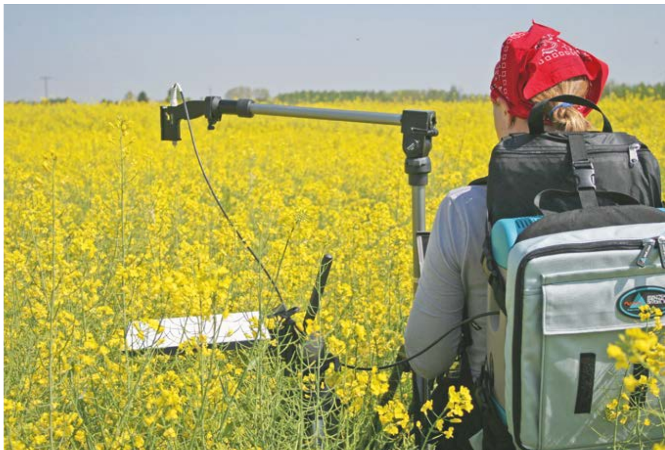
Reflectance measurements in the field: determining the yield and function of rapeseed plants.
