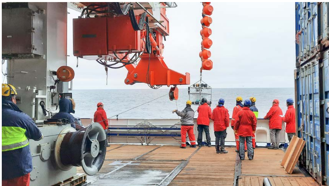
An RAS buoy, which was submerged a year ago, is lifted back on board by a crane.
