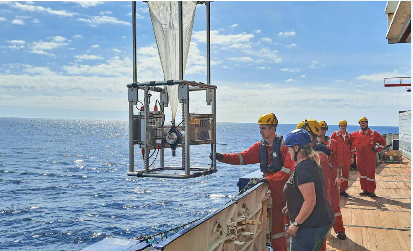
A “LOKI” (Lightframe Onsite Keyspecies Investigation) being lowered into the water. This measuring device photographs microorganisms (zooplankton) underwater. 18 images per second are recorded as it is pulled out of the water. Additional sensors attached to the device measure the oxygen and salinity levels, temperature and pressure in parallel.
